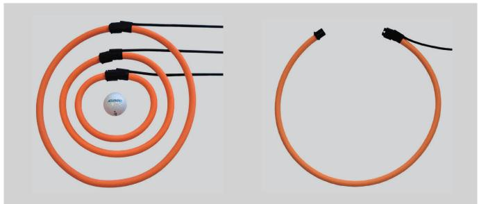
Accuenergy's flexible Rogowski coil is designed for use where regular solid or split core current transformers cannot fit, and is ideal for power quality monitoring such as harmonics. Advantages of the Rogowski coil include; high accuracy, wide measurement and frequency range with no additional integrator or power supply needed.
