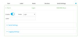
The serial port is enabled by default. To disable, toggle off **Enable**.
